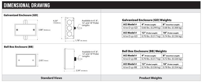
**Note:** There are two enclosures included with configurations involving Temperature Transmitters. A secondary GD (Galvanized) enclosure contains the transmitter board to protect it from the extreme temperatures exposed to the sensing element
